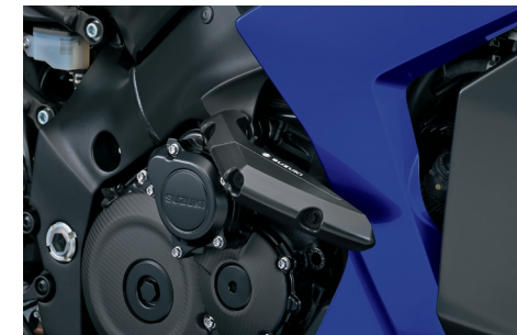
Frame Slider 99114-48K10-000 🇪🇺 Helps reduction of damage, made of aluminum and POM (polyacetal).
