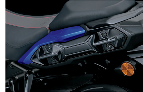
Side Case Bracket Set 93700-48811-000 🇯🇵 For attaching side case set.
